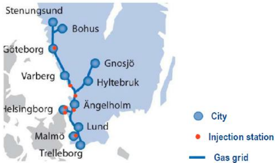
Figure 3- Gas Grid and Locations of Bio Methane Injection Stations in Sweden
