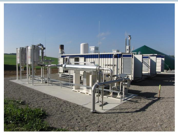
Capacity 500 m<sup>3</sup>/h biogas, 300 m<sup>3</sup>/h biomethane, approx. 8 km pipeline for grid injection and high pressure compression to 60 bar
