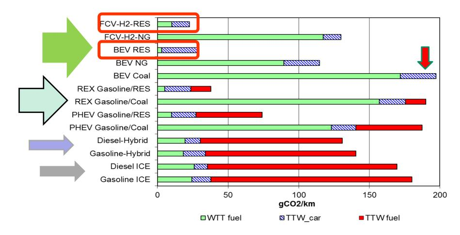
CO<sub>2</sub> emissions per km driven for various types of EV in comparison to conventional cars (power of car: 80kW)
